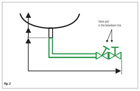
The shut-off valve is often used only in emergencies and usually remains open during normal operation. One of the two valves in this pair must be capable of closing the line slowly. However, either valve must also be able to shut off the line independently of the other, in case one fails. (Fig. 2)
